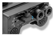
Single mode switch is easy to access and dual remote cable ports add versatility.
