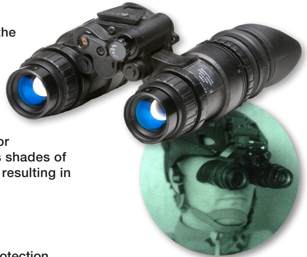
Gen III Night Vision Image Intensifier (I 2 ) Tubes are Available in Green and White Phosphor
